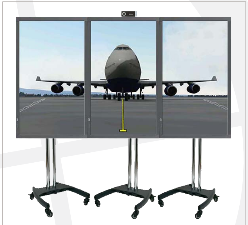
Trainee displays show the high-fidelity 3D airside environment (in this example scenario, a Boeing 747 is approaching a stand).
