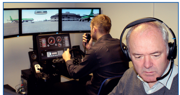
An instructor working with a trainee driver. The instructor has an intuitive touch-screen interface to control background radio conversations.
