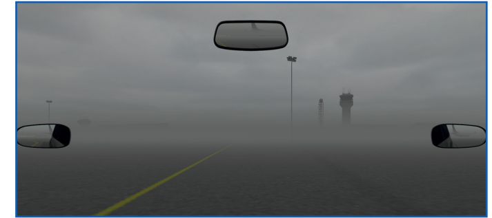
The ADT can simulate adverse weather conditions (rain, snow, fog). This image shows ground fog and reduced visibility, exposing trainee drivers to realistic challenges not practical without the use of simulation.
